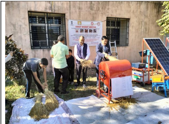
Prof. P. Lingfa (Regional Coordinator, UBA NERIST) demonstrate the Solar power Paddy thresher.
